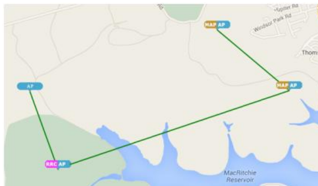
Figure 60: An existing AP is connected to an RRC which is in turn connected to 2 MAPs
